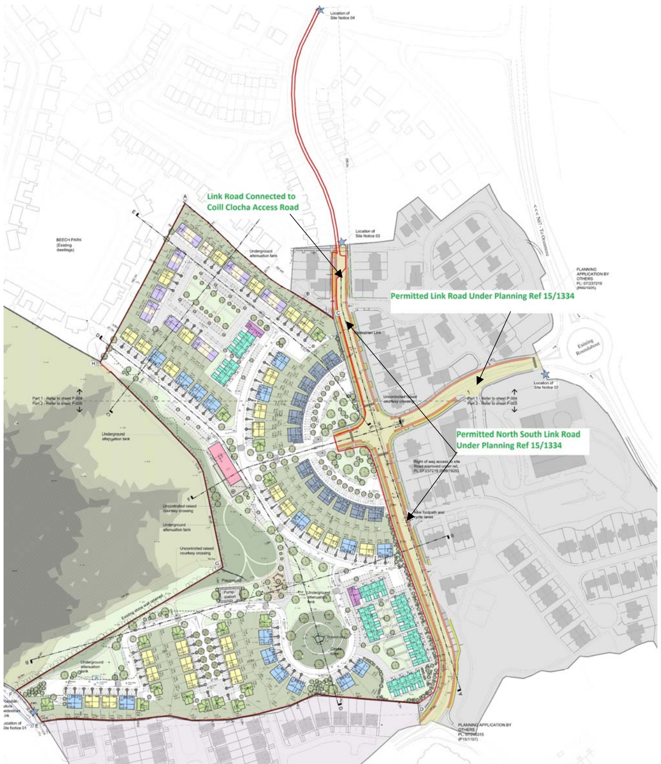
Fig 3.0 – Development showing Link Roads
